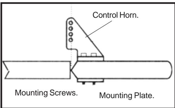
□ 4) Using a 1mm drill bit and the control horns as a guide, drill the mounting holes through the aileron halves.
