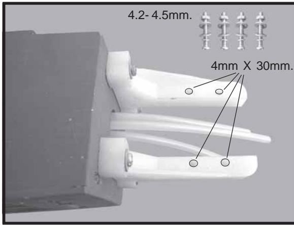
□ 5) Bolt the engine to the engine mount using the four machine screws and lock washer. Double check that all the screws are tight before proceeding.
