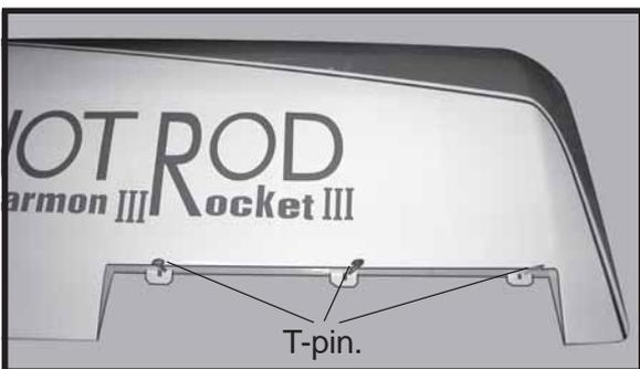
□ 3) Slide the aileron on the wing panel until there is only a slight gap. The hinge is now centered on the wing panel and aileron. Remove the T-pins and snug the aileron against the wing panel. A gap of 1/64" or less should be maintained between the wing panel and aileron.
