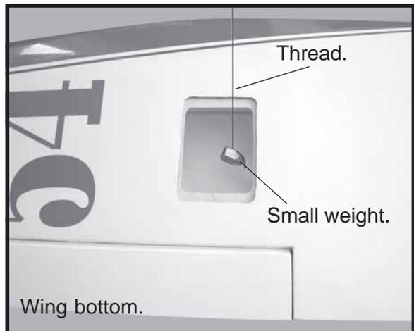
Attach servo lead to the aileron servo. Attach the string to the servo lead and carefully thread it though the wing. Once you have thread the lead through the wing, remove the string so it can use for the other servo lead. Tape the servo lead to the wing to prevent it from falling back into the wing.
