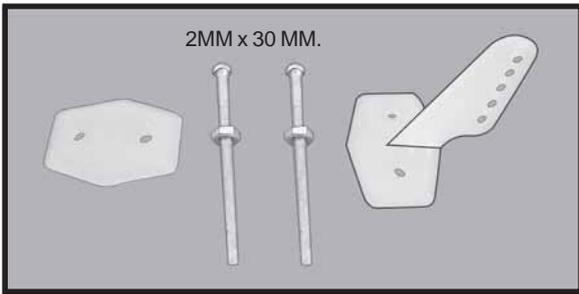
□ 3) Position the aileron horn on the bottom side of aileron. The clevis attachment holes should be positioned over the hinge line.
