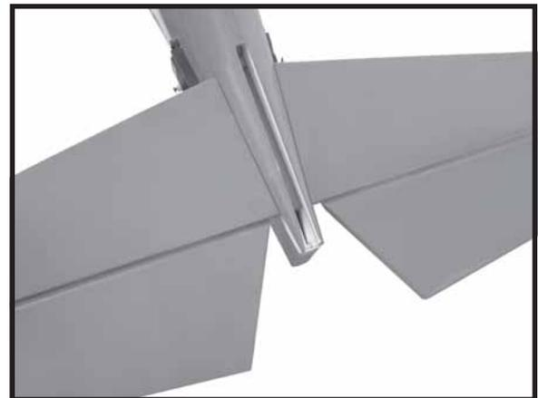
□ 8) After the epoxy has fully cured, remove the masking tape or T-pins used to hold the stabilizer in place. Carefully inspect the glue joints. Use more epoxy to fill in any gaps that may exist that were not filled previously and clean up the excess using a paper towel and rubbing alcohol.
