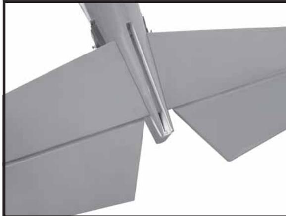
□ 4) With the stabilizer held firmly in place, use a pen and draw lines onto the stabilizer where it and the fuselage sides meet. Do this on both the right and left sides and top and bottom of the stabilizer.
