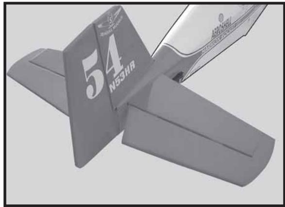
□ 3) While holding the vertical stabilizer firmly in place, use a pen and draw a line on each side of the vertical stabilizer where it meets the top of the fuselage.
