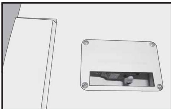
Install the aileron servo tray into the servo mount.
