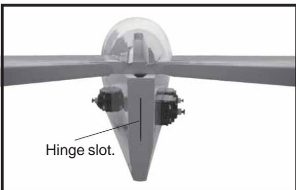
□ 2) Slide the vertical stabilizer into the slot in the top of the fuselage. The rear edge of the stabilizer should be flush with the rear edge of the fuselage and the lower rudder hinge should engage the precut hinge slot in the lower fuselage. The bottom edge of the stabilizer should also be firmly pushed against the top of the horizontal stabilizer.
