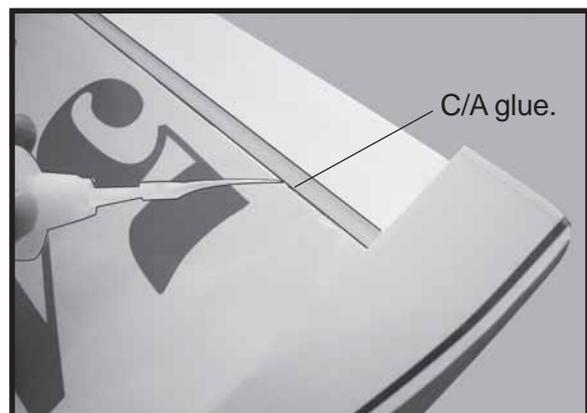
□ 6) Using C/A remover/debonder and a paper towel, remove any excess C/A glue that may have accumulated on the wing or in the aileron hinge area.
