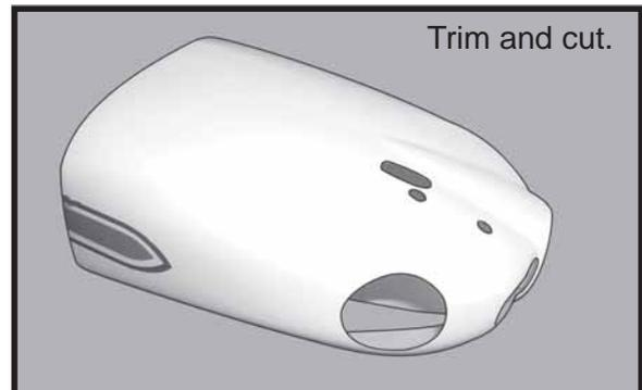
□2) While keeping the back edge of the cowl flush with the marks, align the front of the cowl with the crankshaft of the engine. The front of the cowl should be positioned so the crankshaft is in **nearly** the middle of the cowl opening. Use the spinner backplate as a guide. Hold the cowl firmly in place using pieces of masking tape.
