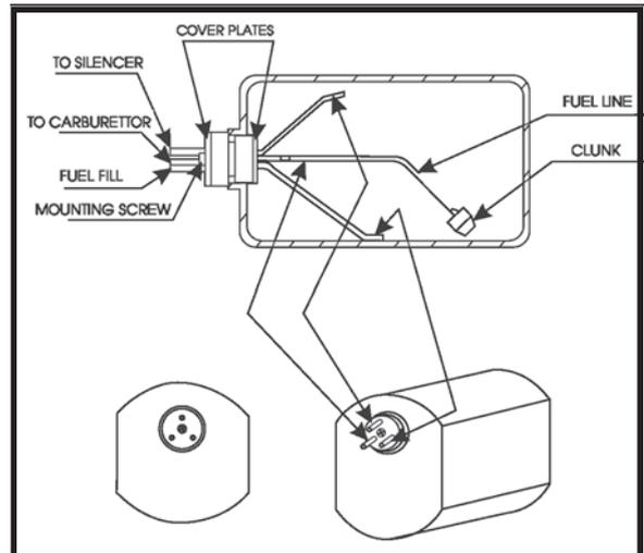
□ 4) Carefully heat the vent tube using a heat gun or lighter to permanently set the angle of the tube.
