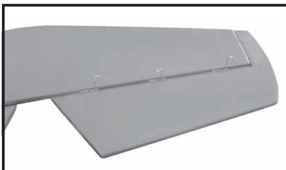
□ 4) Deflect the elevator and completely saturate each hinge with thin C/A glue. The elevators front surface should lightly contact the horizontal stabilizer during this procedure. Ideally, when the hinges are glued in place, a 1/64” gap or less will be maintained throughout the length of the elevator to the horizontal stabilizer panel hinge line.
