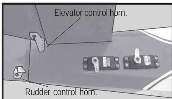
**ELEVATOR - RUDDER PUSHROD INSTALLATION.**
