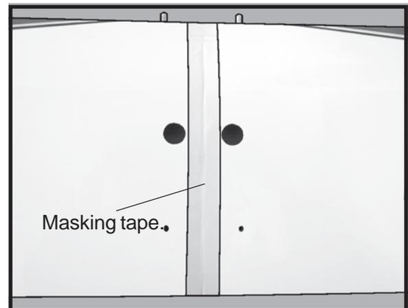
□ 3) Peel off the backing from the self adhesive covering strip. Apply the strip to the centre section of the wing starting from the bottom trailing edge. Wrap the strip all the way around the wing until it meets the trailing edge again. Trim off any excess strip.
