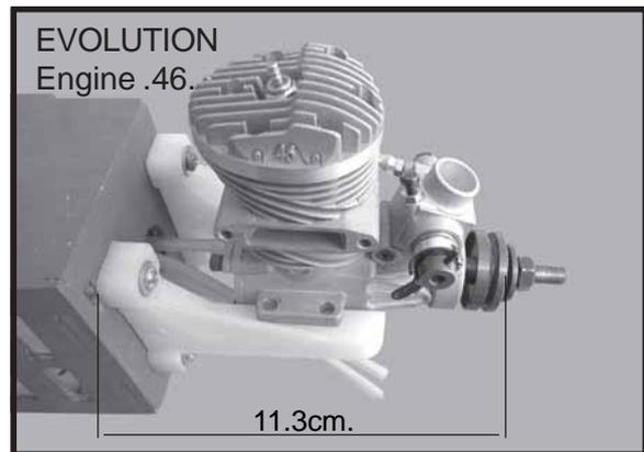
□ 2) Place your engine onto the engine mount. Adjust the engine is centered of the edges of the engine case.
