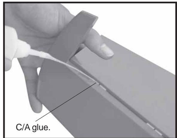
□ 5) Turn the horizontal stabilizer panel over and deflect the elevator in the opposite direction from the opposite side. Apply thin CA glue to each hinge, making sure that the C/A penetrates into both the elevator and horizontal stabilizer panel.
