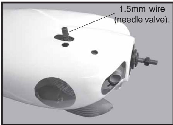
□ 3) Slide the cowl back over the engine and secure it in place using four 3mm x 12mm wood screws. See picture below.
