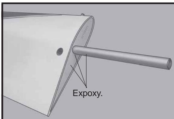
Carefully slide the two wing halves together and firmly press them together, allowing the excess epoxy to run out. There should not be any gap in the wing halves. Use rubbing alcohol and a paper towel to clean up any excess epoxy.
