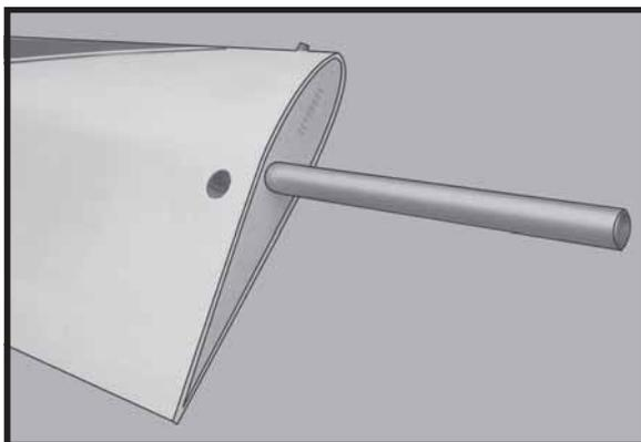
□ 2) Remove the brace when satisfied with its fit in each wing half. Coat both sides of one half of the dihedral brace with 30 minute epoxy. Next, pour some epoxy into the dihedral box in one wing panel. Make sure you cover the top and bottom as well as the sides of the dihedral brace. Use enough epoxy to fill any gaps.
