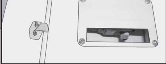
□ 6) Thread one nylon adjustable control horn onto each aileron control rod. Thread the horns on until they are flush with the ends of the control rods.
